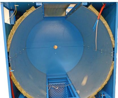
Drying area thermally and acoustically insulated with stone wool
