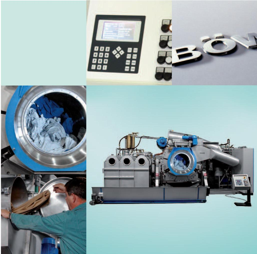
High-capacity drycleaning machine for industrial use
